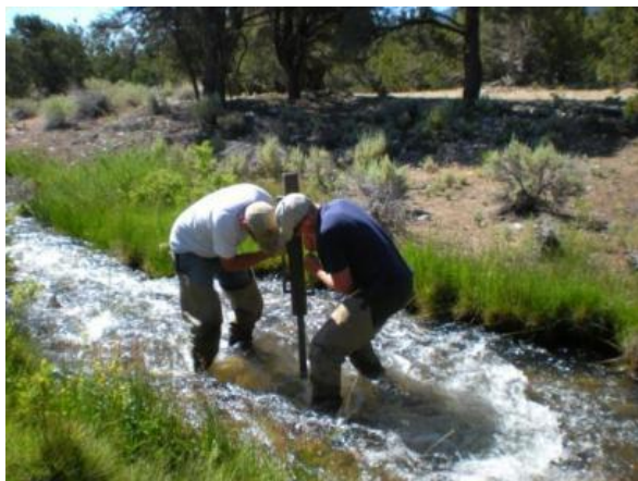
Figure 7. Photograph of well point and pipe being driven into streambed of Lehman Creek east of the Park and near Circle M Ranch Road.
