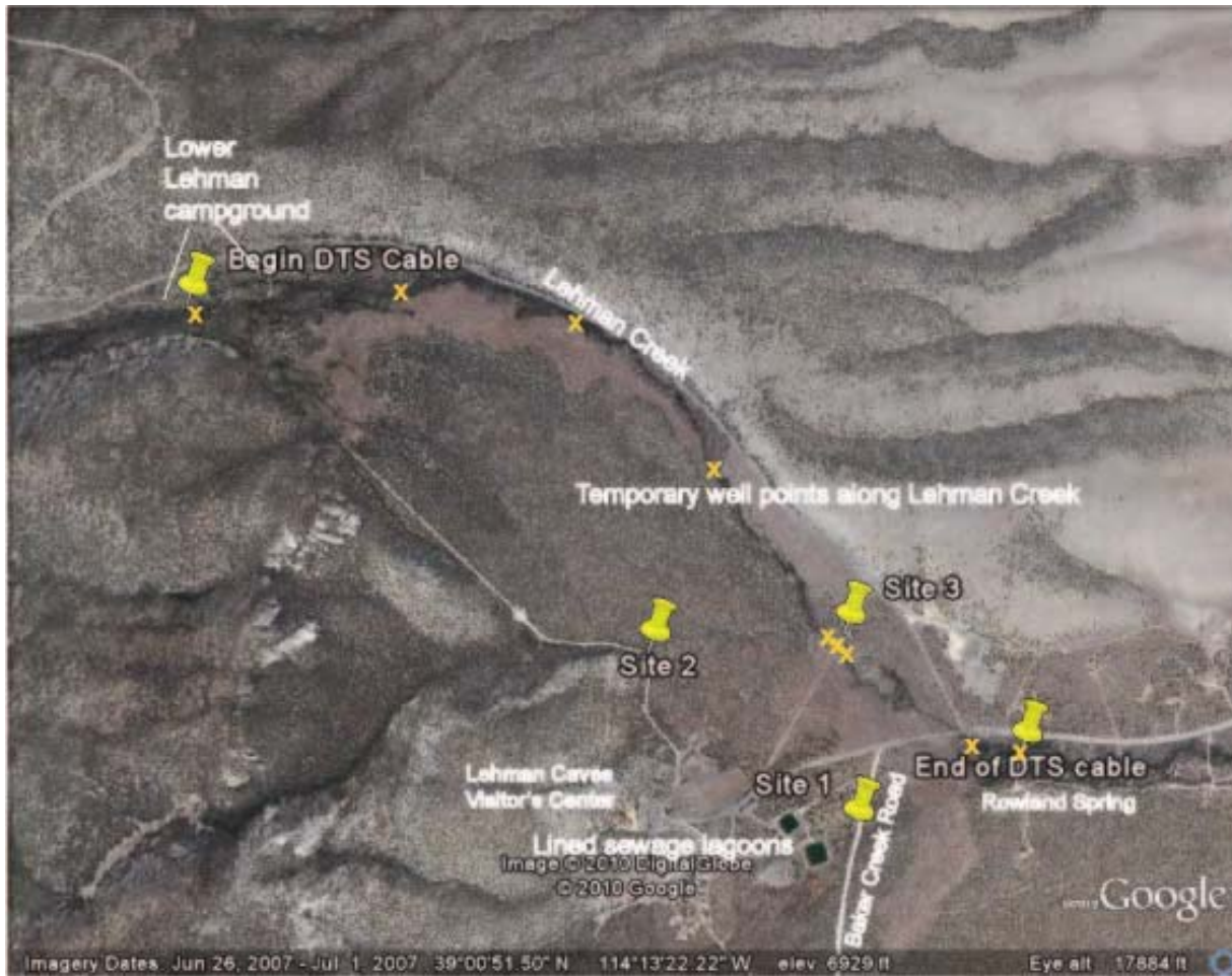
Figure 3. Locations of proposed monitoring wells (sites 1, 2, and 3), extent of digital temperature sensing (DTS) cable in Lehman Creek, and approximate locations of temporary well points along Lehman Creek between Lower Lehman Campground (upstream of contact between quartzite and granite) and Joe's Way just east of park boundary.
