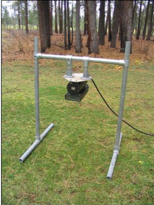
Fig. 2. DIDSON Sonar on an H-mount (CRITFC.org).
