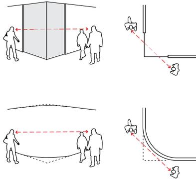
**Figure 5-87.** Wayfinding should be intuitive and clear. Signs should use recognizable pictures. To support movement through the site, use color contrast for identification and transparency to add predictability. Avoid long or hidden corridors (QE, 2020).
