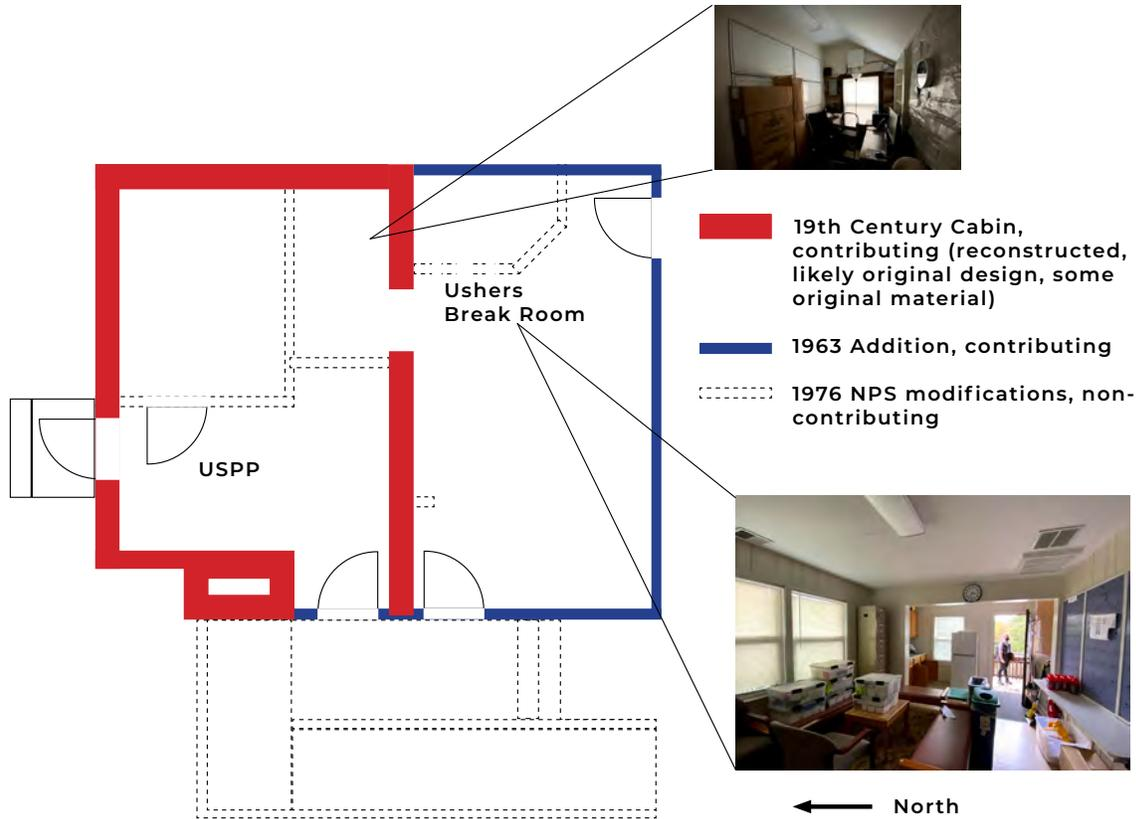
**Figure 6-34.** Existing Cabin floor plan diagram showing era of construction.
