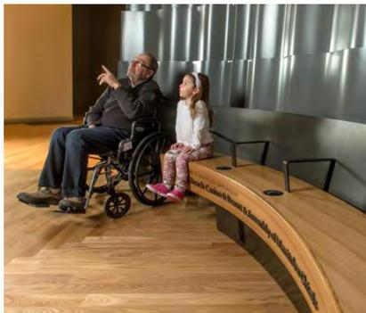
**Figure 5-90.** Integrate seating into the general design of the site. Provide seating for different needs (for example, space for wheelchair users, seating with and without armrests and backs) (QE, 2020).
