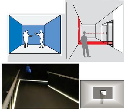
**Figure 5-88.** Lighting should create visual contact for features (lifts, handrails, path edges), and avoid harsh transitions and flickering. Light should be adequate for people to lip read, and for people with partial sight to see information and features. Aim to maximize daylight and wash surfaces with light (QE, 2020).
