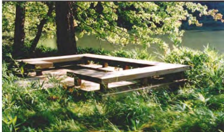
**Figure 6-31.** Example accessible picnic area: low-profile deck with benches.
