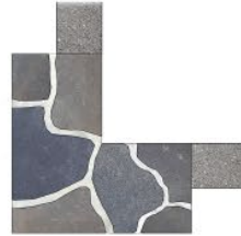
PAVERS - STONE USING STONE SALVAGED FROM THE JAGGAR MUSEUM SMOOTHER STONES WOULD BE USED FOR PAVERS TO PROVIDE AN ACCESSIBLE SURFACE WITH VERTICAL CHANGES IN SURFACE LEVEL NO GREATER AN 1/4"
