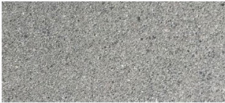
BENCH CAP - CONCRETE BENCHES WILL HAVE A CONCRETE CAP, WITH A LIGHT TO MEDIUM SANDBLASTED FINISH
