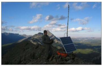
Example of a temporary, or scene-of-action, radio repeater. NPS photo.
