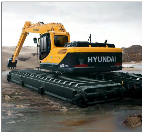
Figure 12 Mitigation of impacts to the saltmarsh will be performed during restoration and will be a direct result of restoration activities. A single piece of heavy equipment will be used on the marsh surface, a low-pressure amphibious floating excavator with 4' wide tracks. The vehicle will move primarily within the footprint of dredge material application. The exception is the southern site where the excavator will access the site either from the road or the tidal creek across approximately 300' of tidal marsh.
