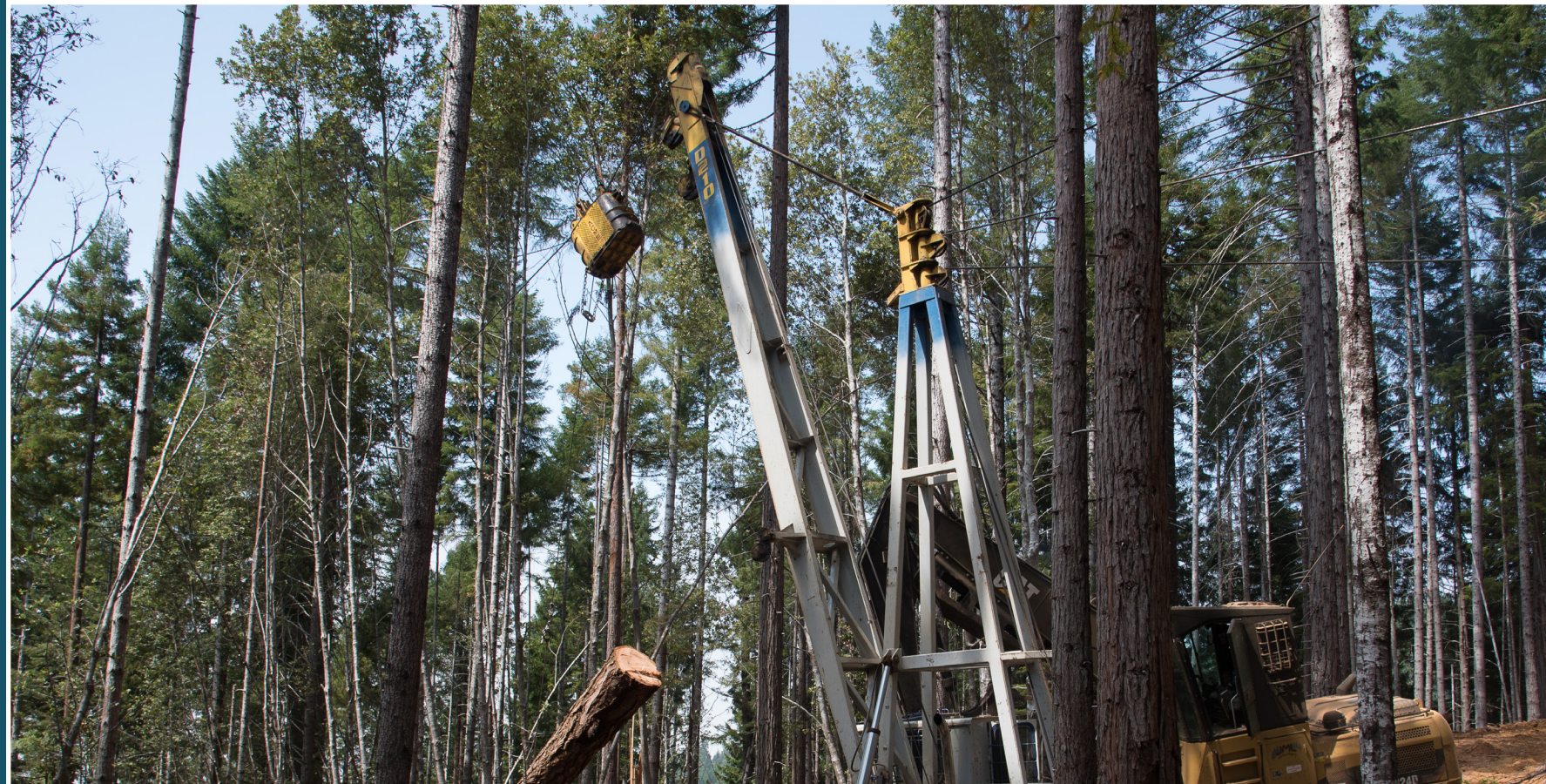
Cable yarding equipment pulls up cut trees on steep slopes to a haul road where they will be removed from the site.
