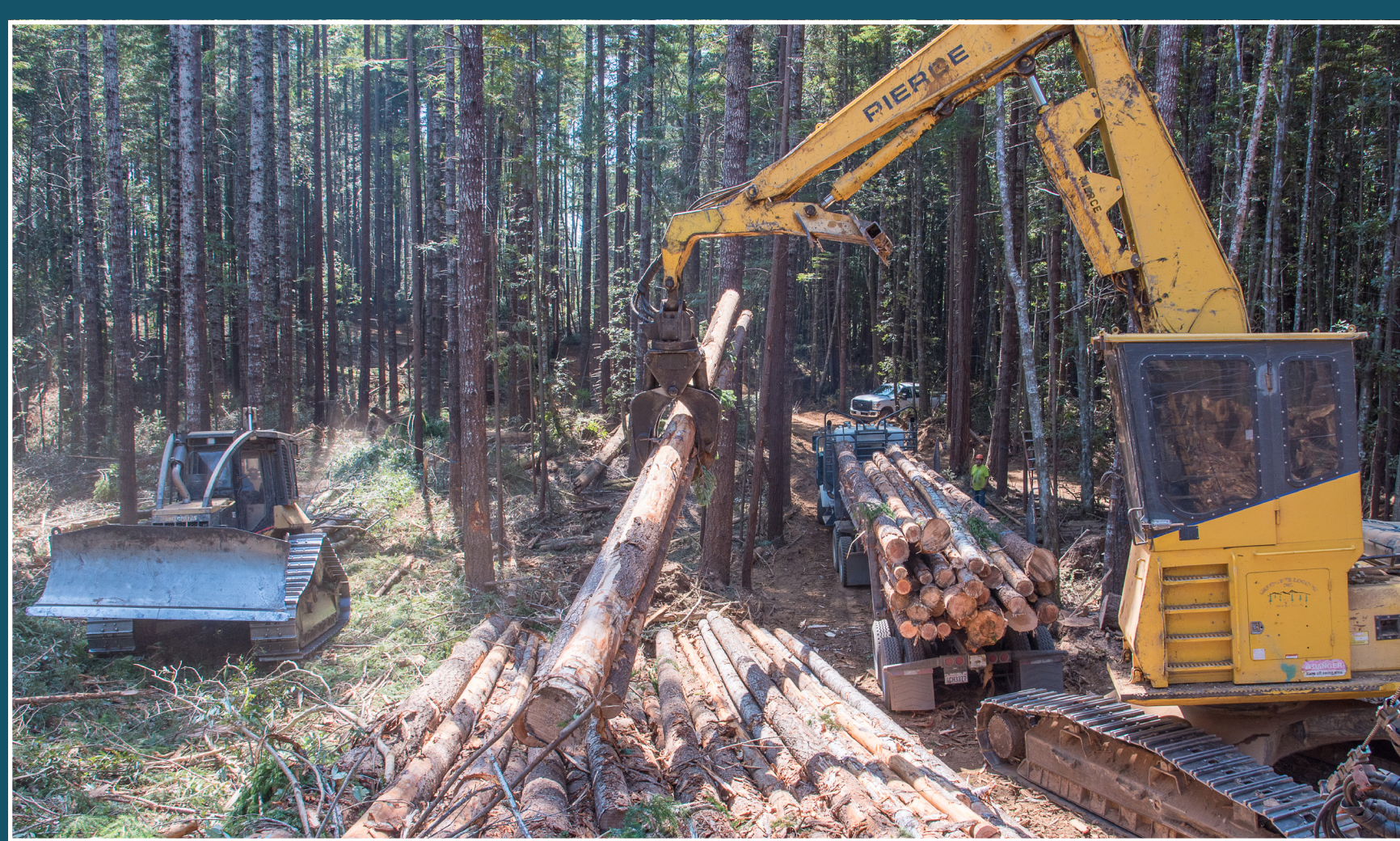
As part of ground-based operations, a skidder pulls cut trees to a small landing, where they are processed and loaded onto a haul truck.
