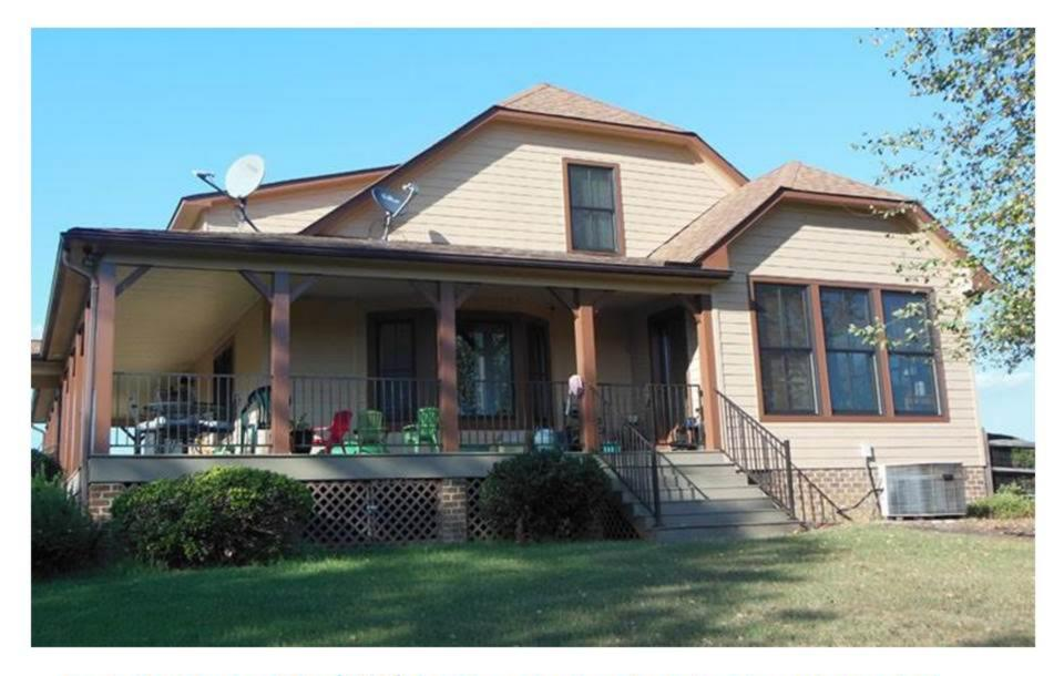
South façade of existing (1996) dwelling, showing clipped-gables and pyramidal porch-roof—and onset of midafternoon shadows of adjacent trees—unsuitable for mounting solar array.
