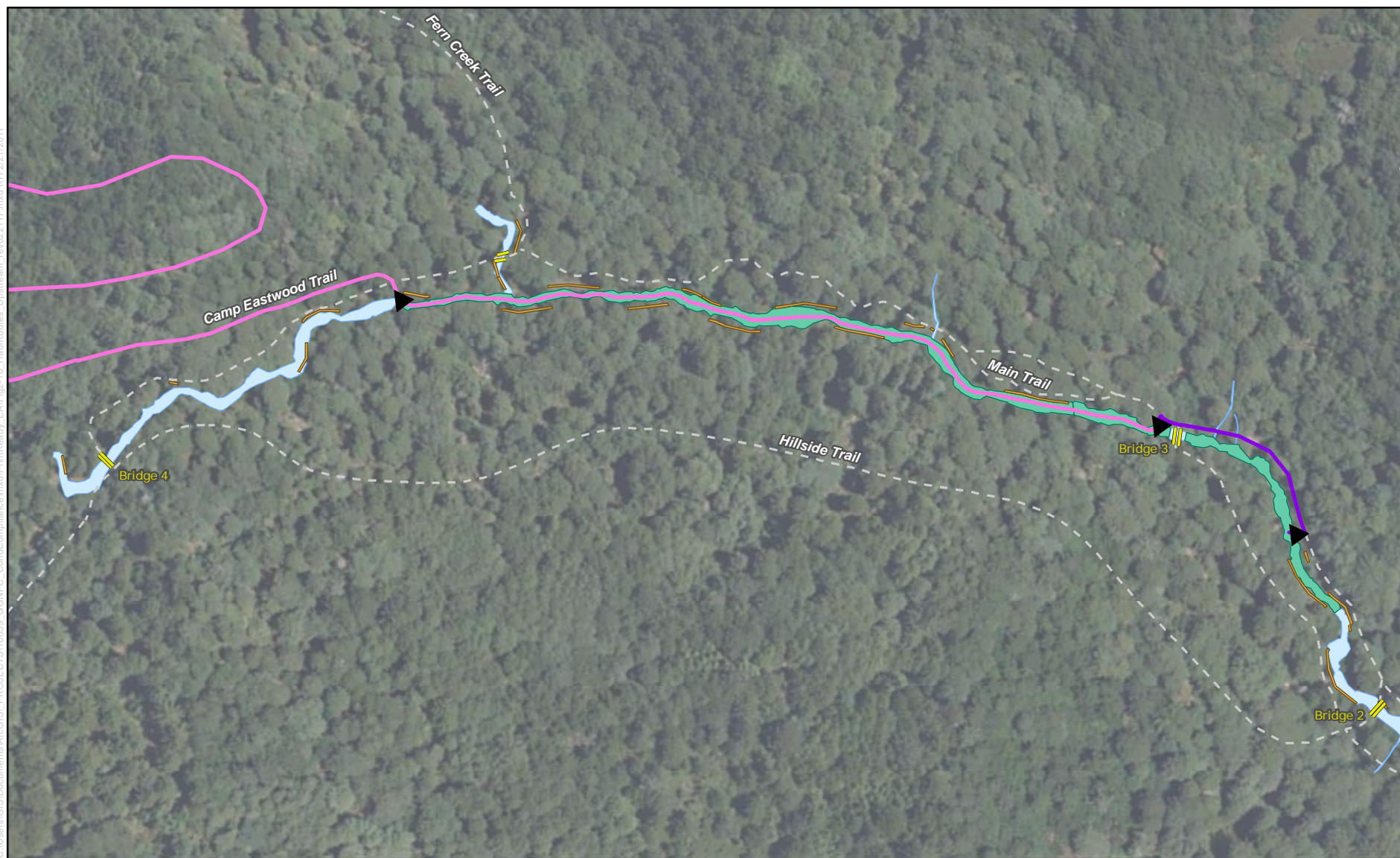
Figure 2-11 Proposed Equipment Access for Riprap Removal Upstream of Bridge 2
