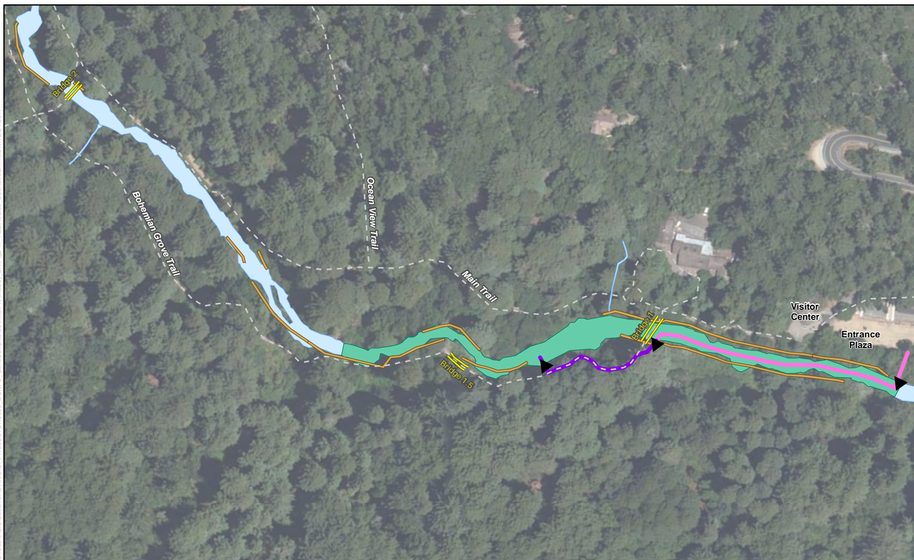
Figure 2-12 Proposed Equipment Access for Riprap Removal Downstream of Bridge 2
