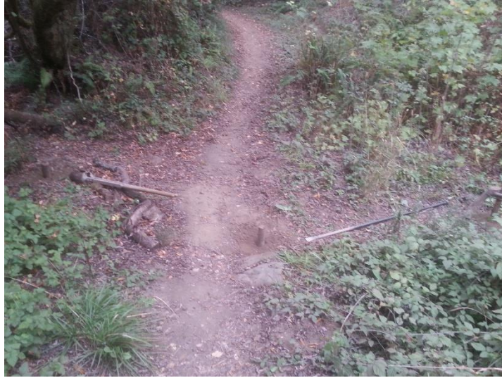
Figure 8. Trail Crossing 1, a stream crossing on Miwok Trail. Displayed in the photo are the investigative digging locations (round posts sticking out of the ground): the trail hole where the digging bar is pointing (photo center), the upstream hole where the post hole digger is pointing, and the downstream hole where the handle end of the digging bar is pointing (far right in the photo). Photo credit: GGNPC
