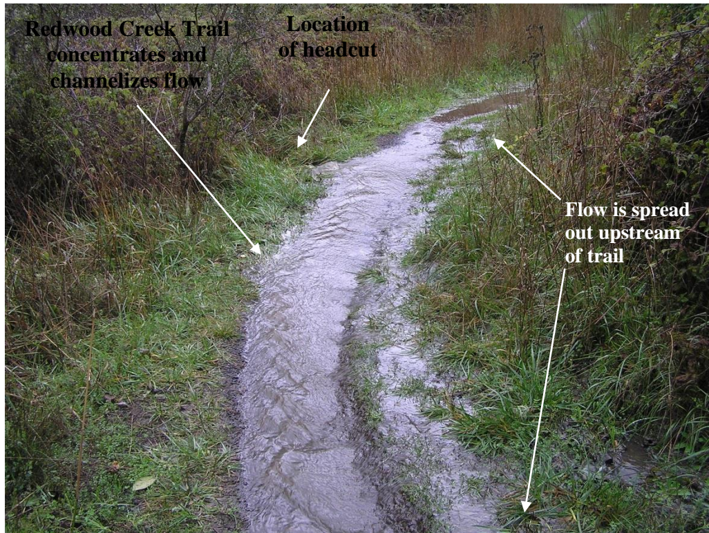
Figure 12. Erosion Site 2 following high rainfall. Water is flowing along Redwood Creek Trail into headcut. Photo credit: GGNPC
