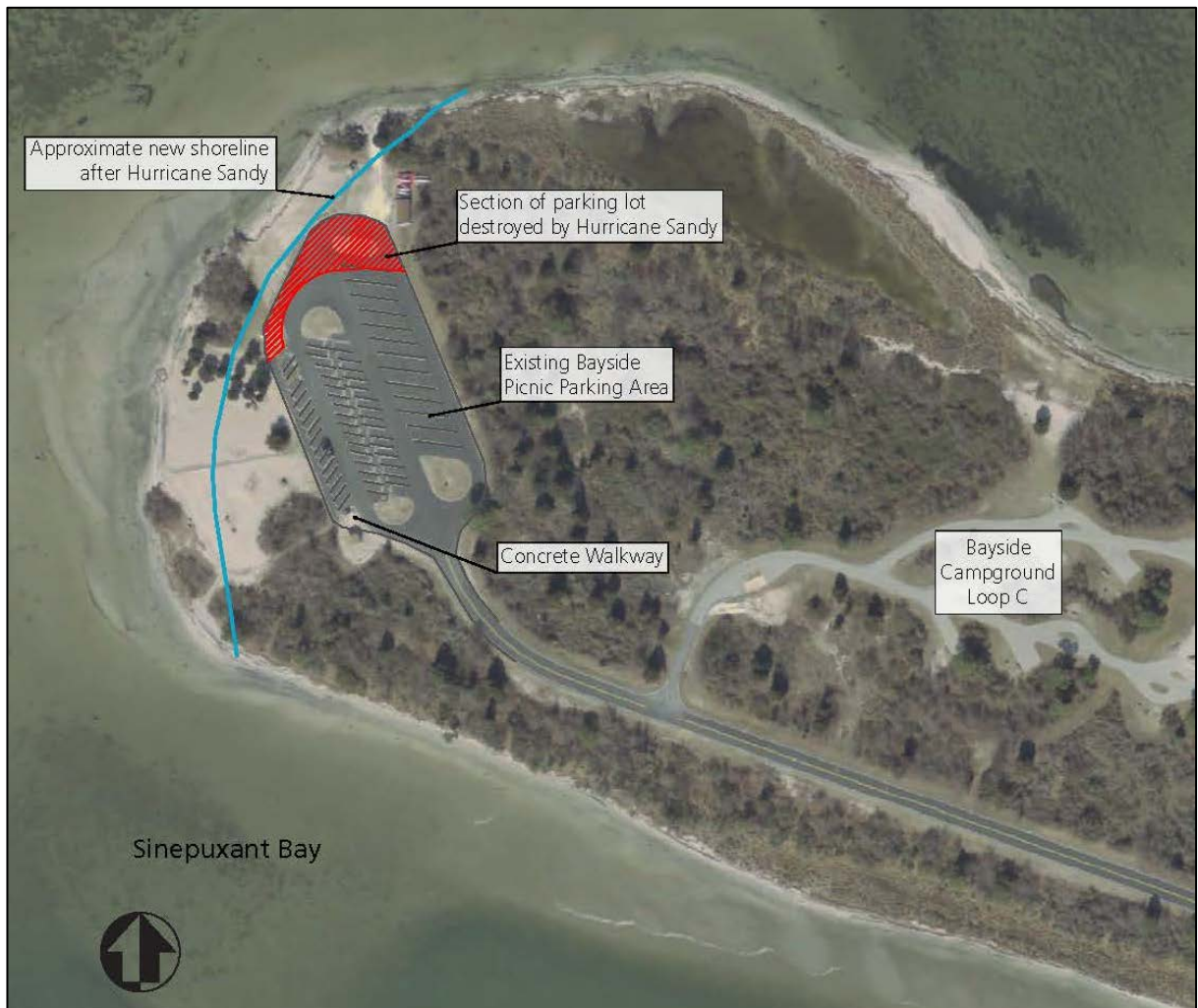
Figure 3: Shoreline and asphalt encroachment at the Bayside Picnic and Parking Area resulting from damage sustained during Hurricane Sandy
