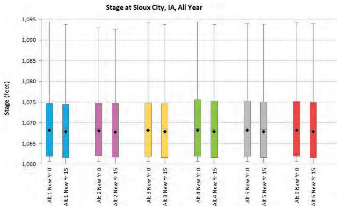
Figure D-25. Comparison of Stages between Year 0 and Year 15 for Sioux City, Iowa, under Alternatives 1 to 6 over the Period of Record (mean, median, and 5th and 95th percentiles)
