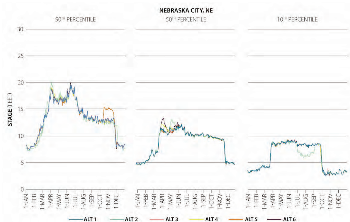
Figure D-16. Stage of the Missouri River at Nebraska City, Nebraska, under Alternatives 1 to 6 over the Period of Record (90th, 50th, and 10th percentiles)
