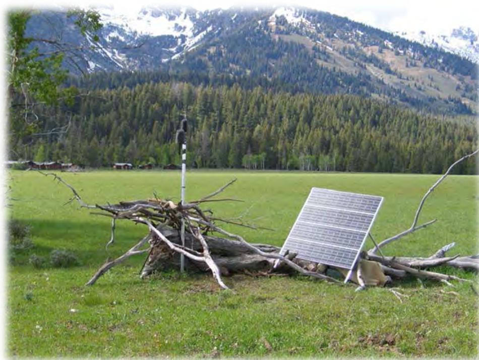
FIGURE 21. THE WHITE GRASS SOUND MONITOR, THE MICROPHONE PROTECTED FROM CURIOUS ELK (FEBRUARY 2004–FEBRUARY 2005)
