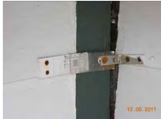
Figure 3-123: Separation of west wing from center of house as measured by crack monitor installed in 2004, PD 12/6/11
