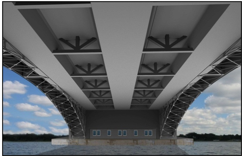
Figure 58: Conceptual rendering of the concrete box girder replacement structure proposed under Alternative 1A (Underside View)
