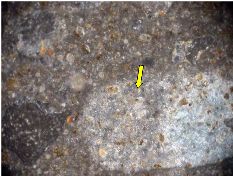
Figure 7. A cement lump in the mortar is marked with an arrow. Note the variable density in the lump, which may be related to internal differences in w/c. Note that the lump is lighter in color than the surrounding (probably pigmented) mortar. The photo was taken using reflected light. The width of the field of view is 1.0 mm.
