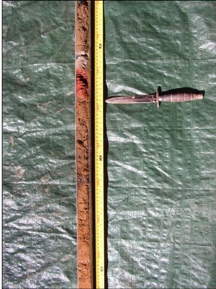
Figure 1. The increment of the Boring 5 soil profile containing an apparently mostly intact original surface at the depth of 6.5 ft just below a large brick fragment. The surface had likely been plowed, and may also have undergone minor grading.
