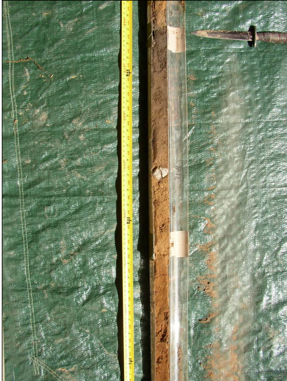
Figure 4. Increment of the Boring 15 profile showing the buried surface at the depth of 21.7 ft. The visible break in the gravel below the plow zone is due to sampling, but a much older break is on the underside.
