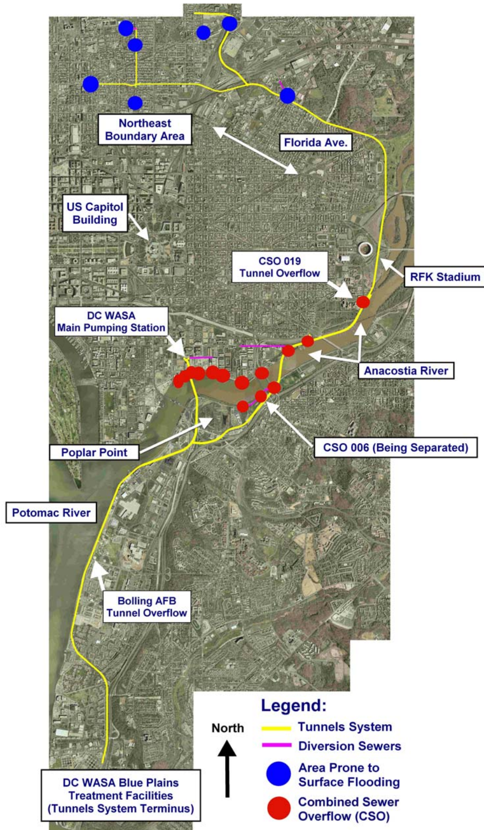
Figure 2: Location of Tunnels System Relative to CSOs and Flooding Areas
