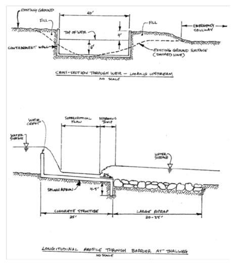
**Figure G-8.** Cross-section through weir (upper diagram) showing elevation of existing abandoned roadbed (existing ground) and longitudinal profile (lower diagram) showing location of splash apron extending 25 ft along stream bottom from the base of the weir.
