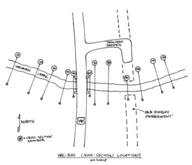
**Figure G-7.** Location for construction of a permanent fish barrier on Specimen Creek in Yellowstone National Park. The barrier would be placed at cross-section #90 and between the abandoned HWY 191 road embankment, just upstream of the existing HWY 191 road bridge.
