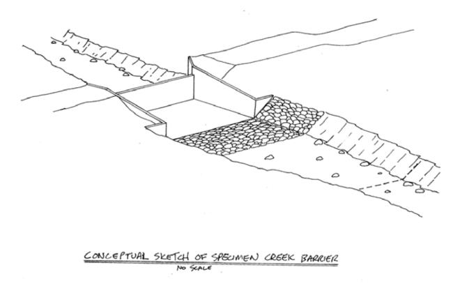
**Figure G-9.** Conceptual sketch of the fish barrier to be constructed on Specimen Creek, a tributary of the Gallatin River, in Yellowstone National Park. View is from below (downstream of) the barrier looking upstream to show the concrete splash pad at the base of the barrier.
