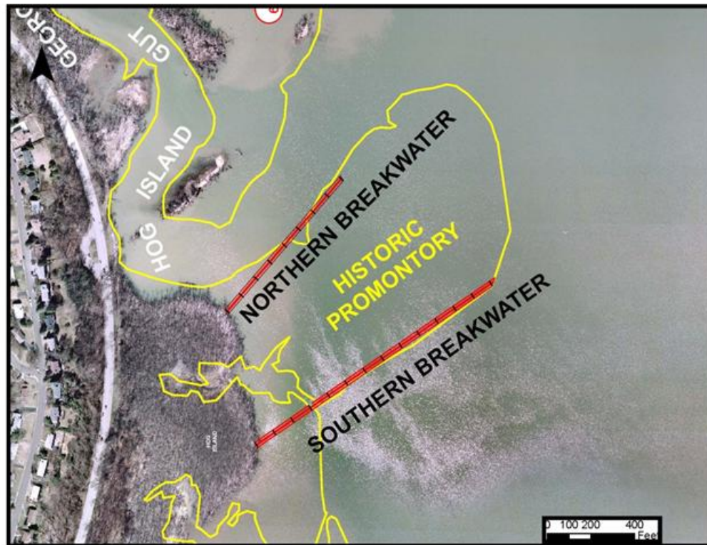
FIGURE 2-1. PLACEMENT OPTIONS FOR THE BREAKWATER STRUCTURES
