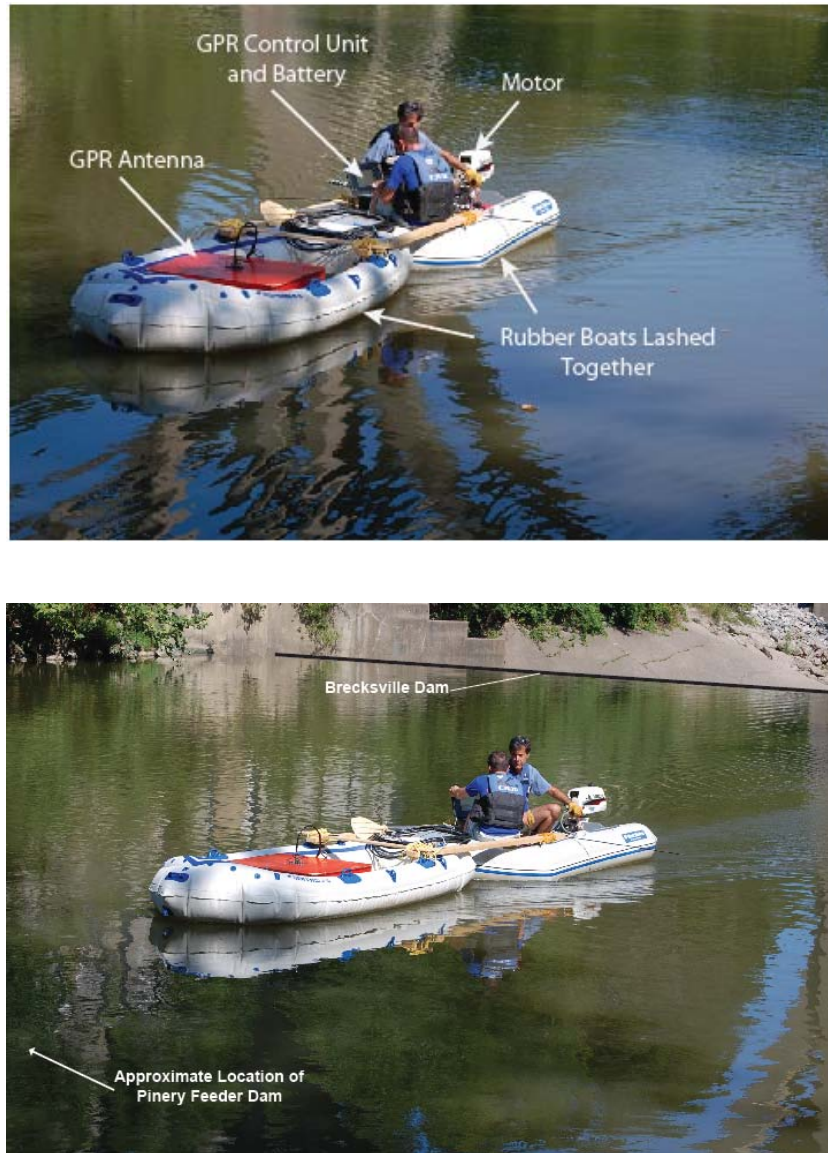
Figure 3. (Top) Photograph of the GPR survey. Two rubber boats were lashed together to allow for separation of the antenna from potential interference by the motor, battery, GPR control unit, and cables. The 120 MHz antenna was placed by itself in the front boat. (Bottom) Photograph showing the measurements of a GPR survey trackline, location of the Brecksville Dam and approximate location of the Pinery Feeder Dam. Photos by Greg Tkachyk.
