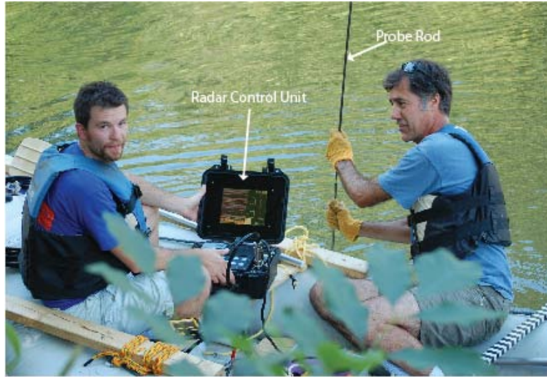
Figure 5. Photograph showing the method of determining a site specific dielectric constant by physically measuring the water depth while simultaneously collecting GPR data. Photo by Greg Tkachyk.
