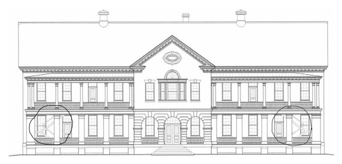
The new, fire egress stairs are visible only behind the main structure and detailing of the building. They are painted to blend in with the shadows of the porch.
