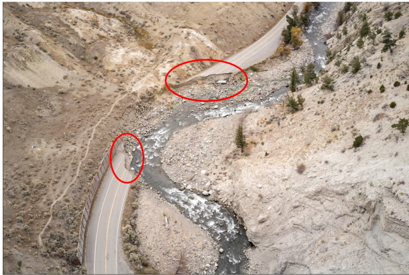
Photo 8. Overhead view of Gardner River Canyon post-2022 flood (source: NPS). Bank stabilization and riparian buffers (red circles) in select locations would enhance the Gardner River and fringe wetlands.
