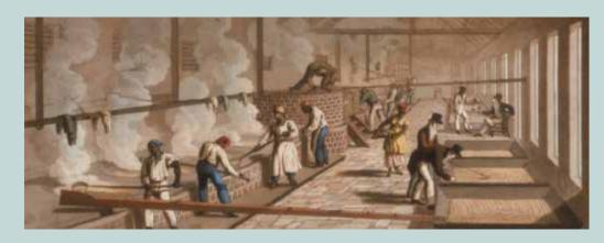
A period drawing showing the process of boiling, skimming, and cooling of sugar in a factory (St. Croix Landmarks Society).
