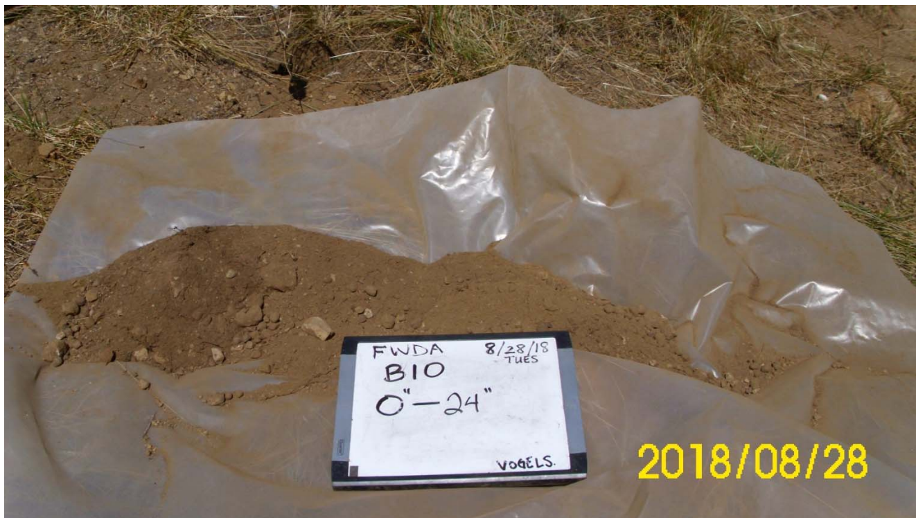
Photo 8: Borehole 10 beyond the extent of debris. Refusal on bedrock at 2 feet bgs.
