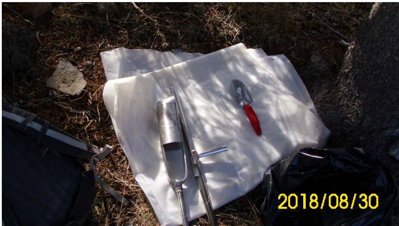
Photo 10: Decontaminated equipment including hand auger, step sampler, and trowel on clean visqueen. Date: 8/30/2018 8:46AM
