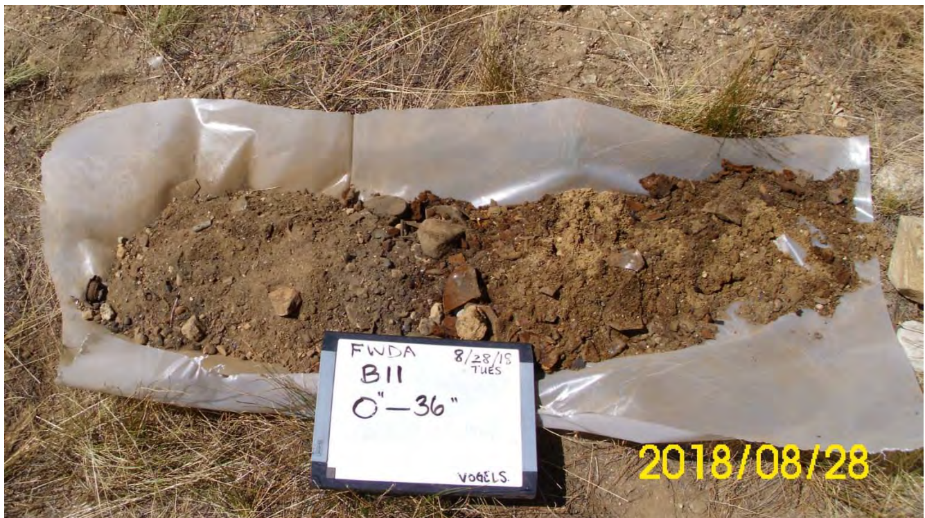
Photo 6: Borehole 11 extent of debris. Refusal at 3 feet bgs.
