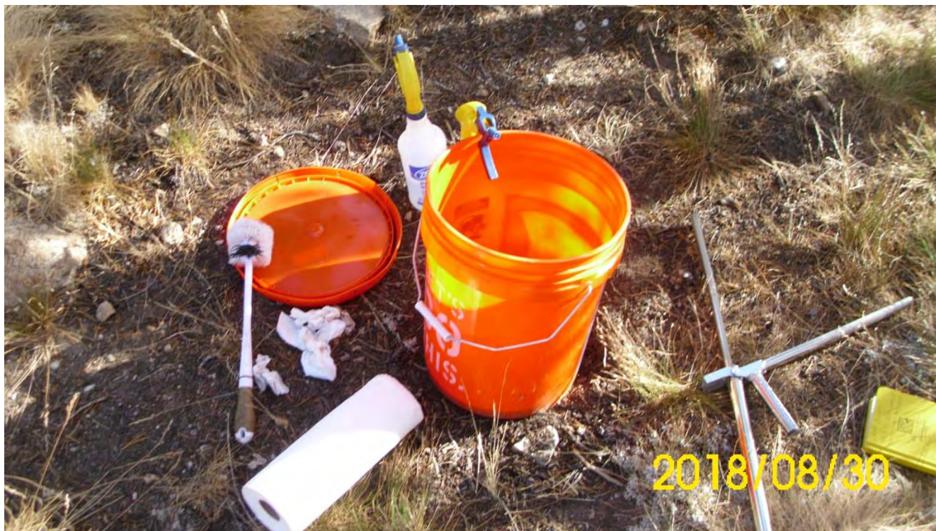
Photo 9: Decontamination materials including alconox spray, rinse water, scrub brush, 5-gallon bucket, and paper towels. Date: 8/30/2018 8:46AM
