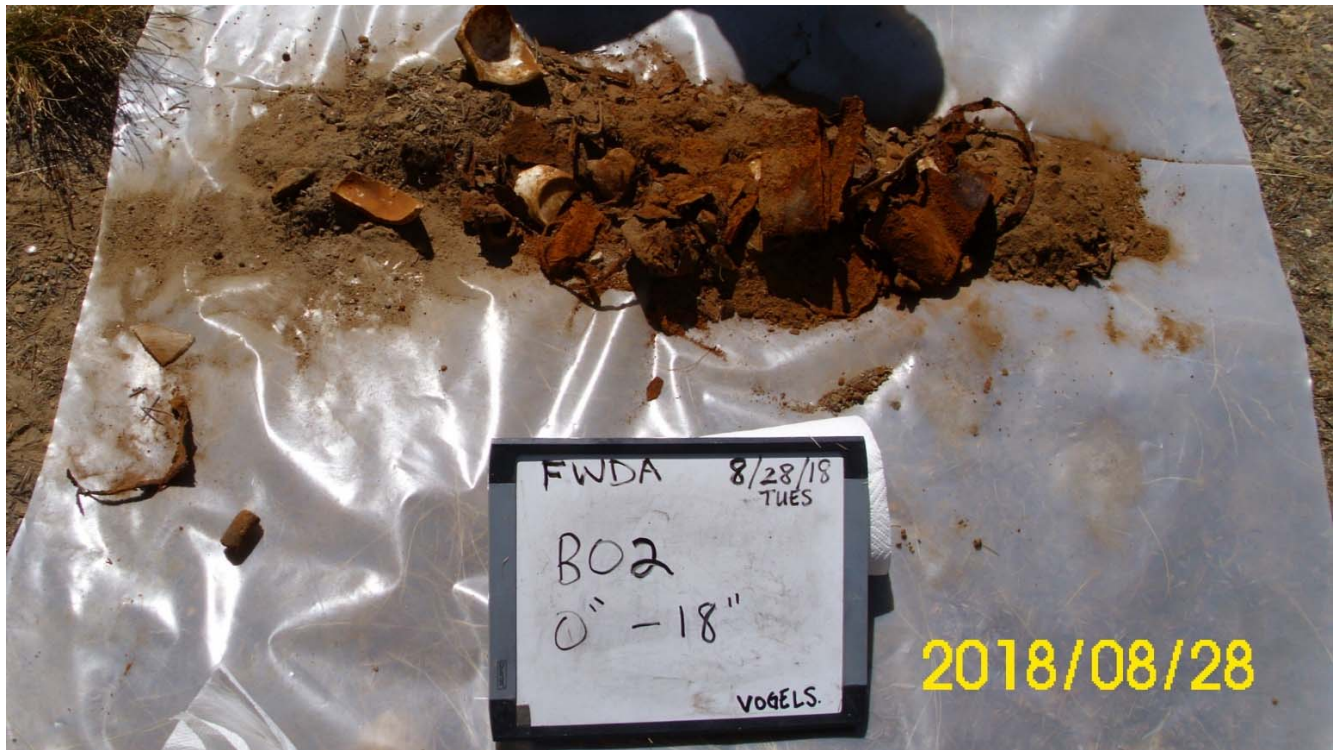
Photo 5: Borehole 02 extent of debris. Refusal at 18 inches below ground surface (bgs).
