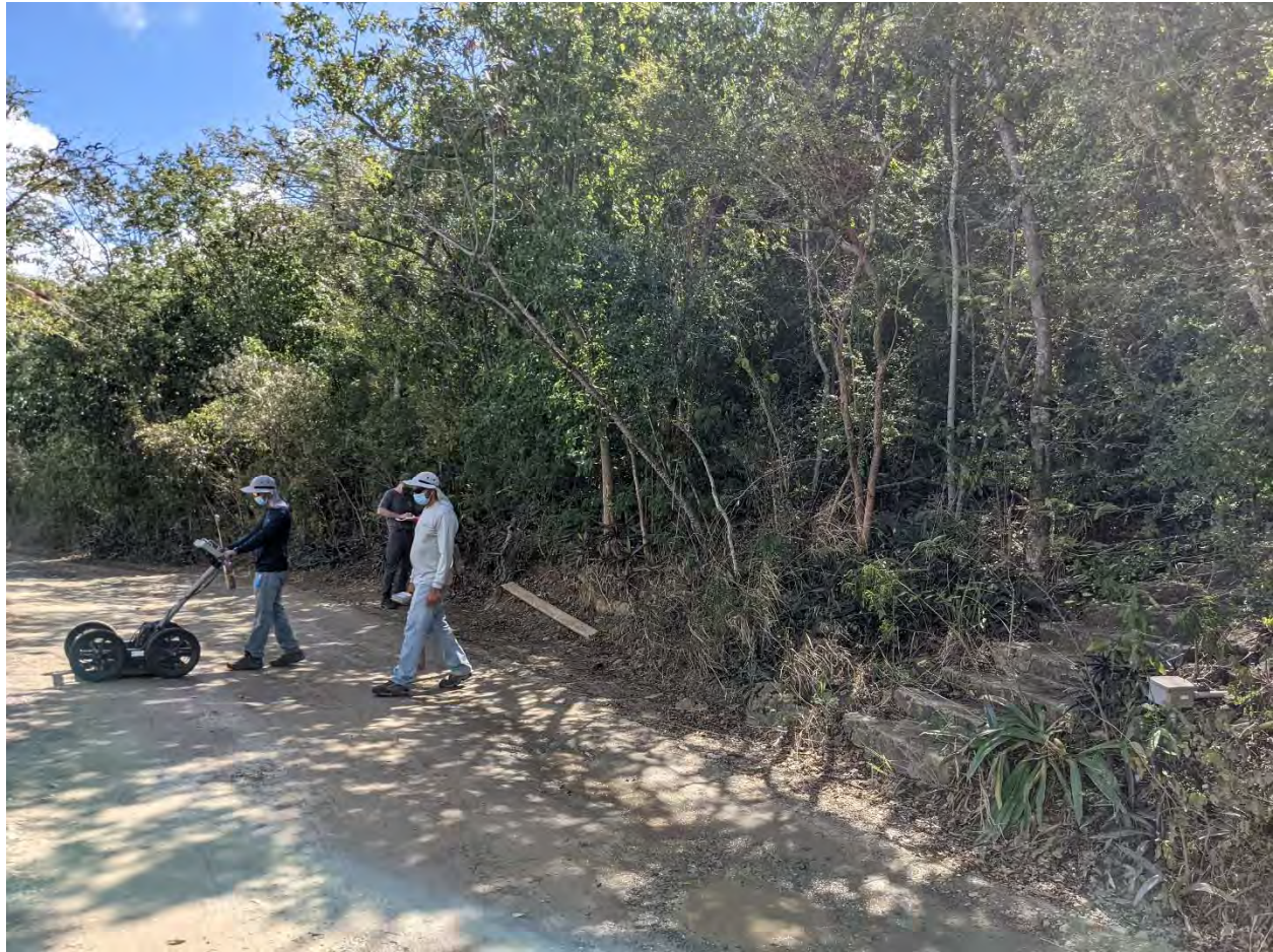
Photograph 3. View of subsurface utility clearance using GPR and EMI of proposed drilling location along access road to Honeymoon Beach.
