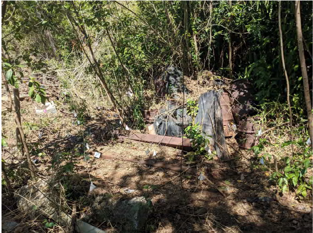
Photograph 7. View of at least 12 partially buried, rusted drums observed in eastern portion of Area 1. The drums contained washed gravel. VHB defined surface soil decision unit IA-1-03 to encompass this area.
