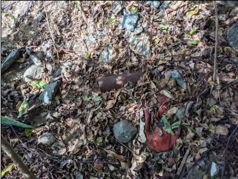
7. Possible asbestos pipe at the southern end of the gravel staging area
