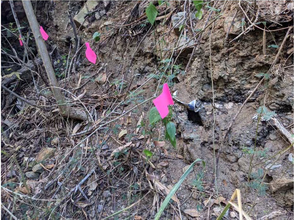
Photograph 8. View of exposed waste (including aluminum, steel, plastic, building materials, and unknown organic material) along the landfill's southern face and apparent seeps. VHB defined surface soil decision unit IA-3-04 to encompass the seep area and characterize potential contaminant migration to the apparent wash.
