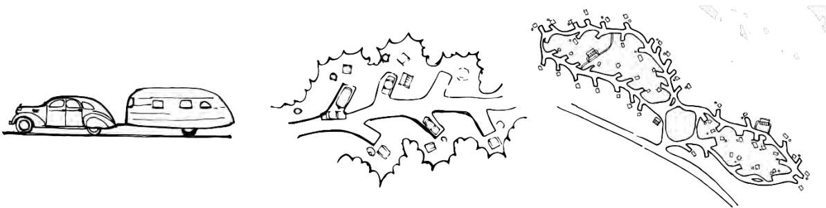
Figure 1.4 1930s to 1940s. The loop campground roads with parking spurs is a signature of 1930s "Meinecke System." The system included one-way loop campgrounds with parking spurs; rustic style picnic tables and fire grates at every campsite; group amenities provided, including comfort stations, picnic areas, fire rings and water spigots.
