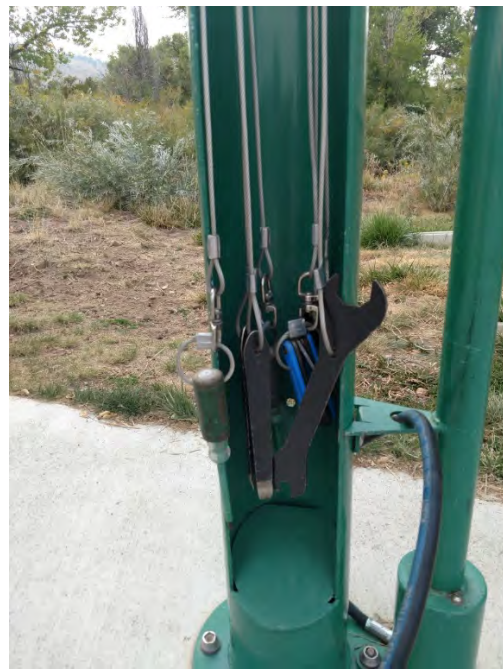
Figure 3.12 Consider adding a fixed bike tool stand like this one at a park in Jefferson County Colorado. The photo on the right shows a close up of tools attached to cables. The stand also includes a tire pump.
