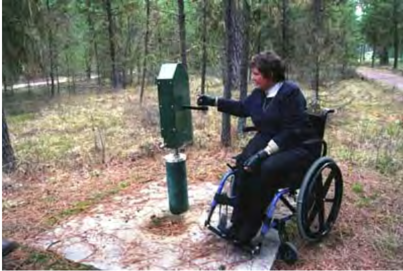
Figure 3.66 Accessible handpump system. Photo courtesy of USDA US Forest Service.
