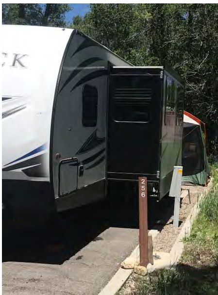
Figure 3.83 Many camper pop-outs are located on the same side as the utility hookups. For this reason, additional protection is needed to prevent a camper for inadvertently damaging utilities.
