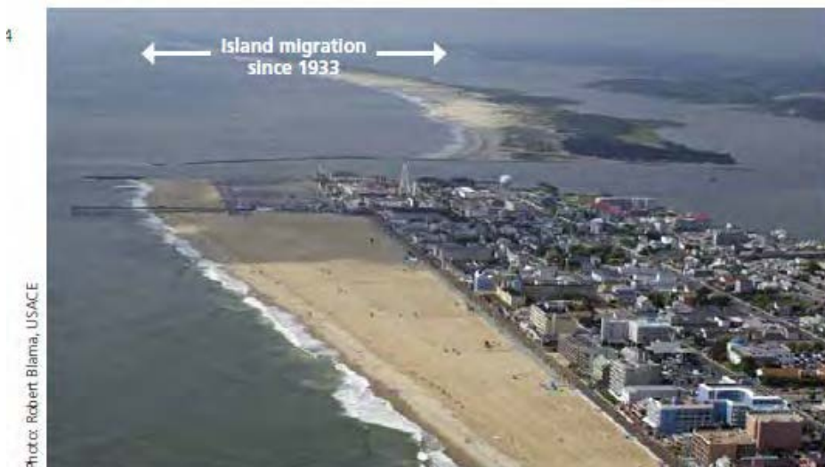
Figure 3.4 Accelerated erosion caused by jetties, groins, and other efforts to stabilize the Ocean City Inlet (particularly at the northern end Assateague Island) (photo taken in September 2004)
