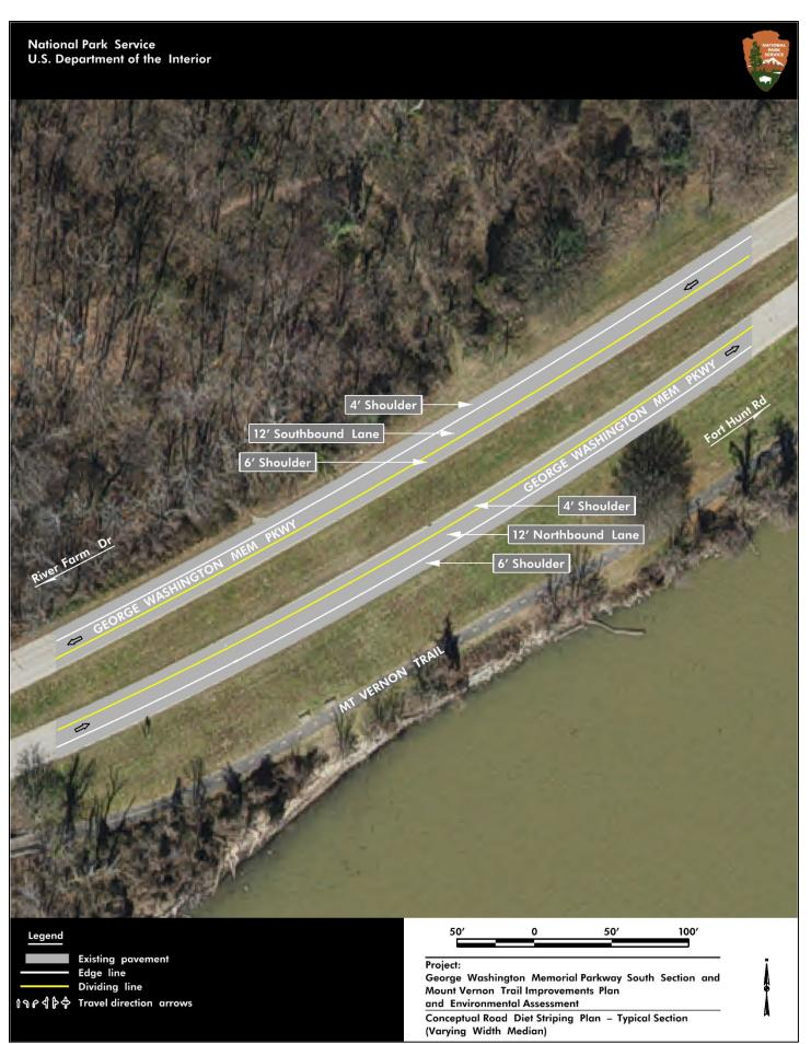
Figure 2. Conceptual Road Diet Striping Plan – Typical Section (Varying Width Median)
