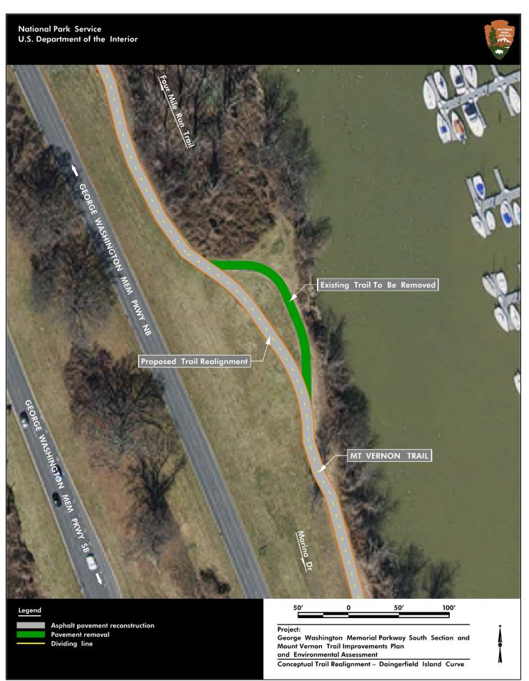
Figure 15. Conceptual Trail Realignment – Daingerfield Island Curve
