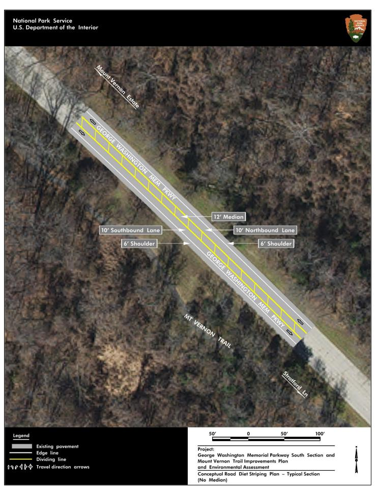
Figure 1. Conceptual Road Diet Striping Plan – Typical Section (No Median)
