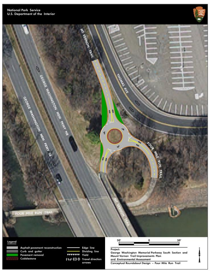
Figure 16. Proposed Roundabout Design – Four Mile Run Trail
