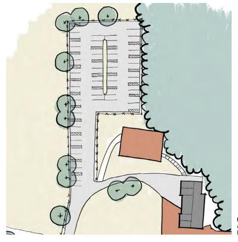
**Figure A-9.** A total of 57 accessible parking spaces could be located within Lot 3 (QE, 2020).
