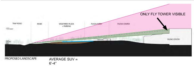
**Figure A-3.** Grading for parking within the dimple and the height of cars within this space would block views of all but the Filene Center fly tower from the Main Circle Drive (QE and Gensler).
