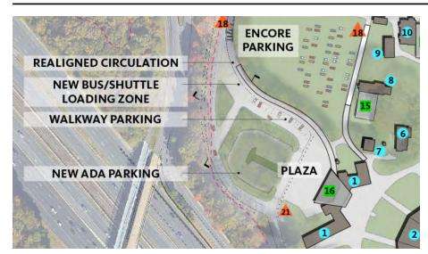
**Figure A-1.** Conceptual plan for parking within the dimple (Gensler, 2020).
