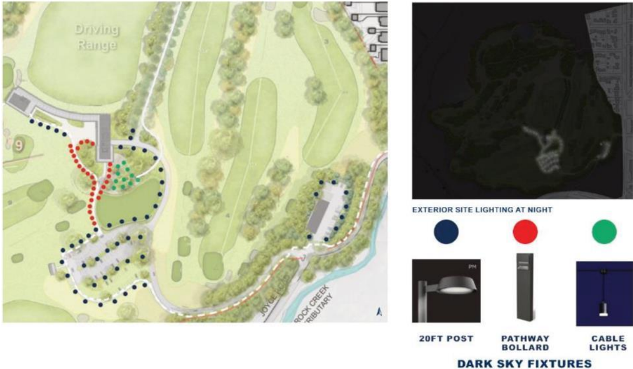
Figure 6. Exterior Site Lighting Plan
