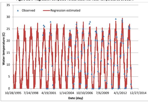
Figure B14. Regression computed versus observed water temperatures at BC14.
