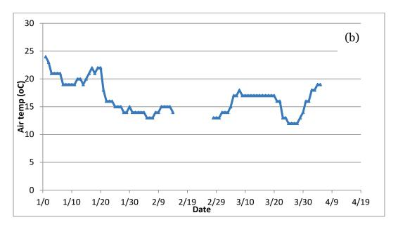
All gaps in meteorological data obtained from the above stations were linearly interpolated in HEC-DSS in order to use them as model inputs. Thus, the data gaps were filled with a straight line between the two bounding values. All meteorological data (after filling gaps) were compiled into one single HEC-DSS file (MoRmet.dss). For example, Figure 6 shows the time series plot of hourly air temperature at the Columbia Regional AP, MO station.
