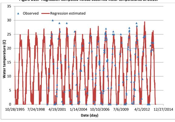
Figure B16. Regression computed versus observed water temperatures at BC16.
