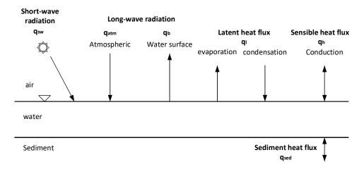
Units of heat flux (W m<sup>-2</sup>) are used to describe heat exchange at the airwater and sediment-water interfaces. The sign convention used herein is positive (+) for heat entering the water column, and negative (-) for heat leaving the water column. Net heat flux ( $q_{net}$ ) for the water column is
