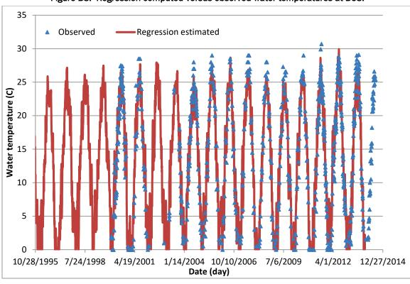
Figure B8. Regression computed versus observed water temperatures at BC8.
