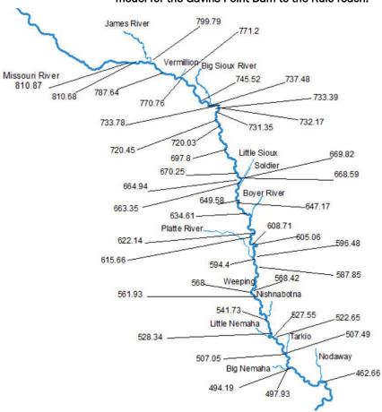
Figure 29. Schematic representation of inflow boundary locations included in the HEC-RAS model for the Gavins Point Dam to the Rulo reach.
