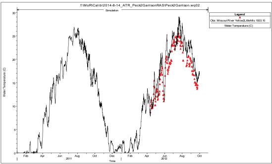
These figures show a scatter plot of instantaneous temperature predictions against time-stamped temperature observations. Comparisons of model predictions and observed data at USGS stations along this river reach demonstrate the degree that the HEC-RAS model captures the
