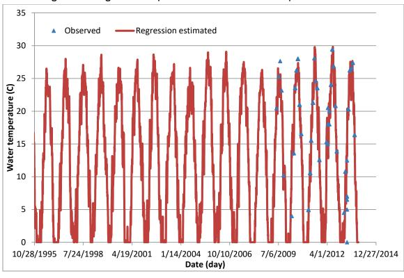
Figure B10. Regression computed versus observed water temperatures at BC10.
