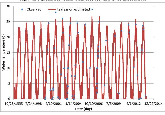
Figure A8. Regression computed versus observed water temperatures at BC8.
