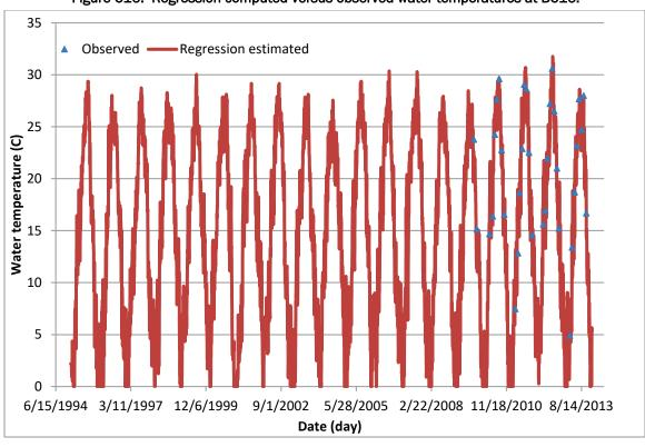
Figure C16. Regression computed versus observed water temperatures at BC16.
