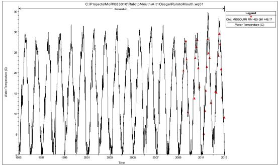
Figure 42. HEC-RAS predicted versus observed water temperatures of the Missouri River at Kansas City, MO (USGS 06893000).
