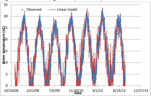
Figure 8. Observed vs. linear-regression-computed water temperatures at USGS 0689300.
