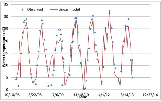
Figure 10. Observed vs. regression-computed water temperatures at USGS 05587455.
