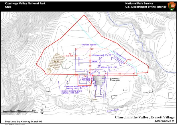
Figure 15. Schematic Drawing of Alternative 2 showing general location and layout of parking lot and septic system. See Appendix D for full version.
