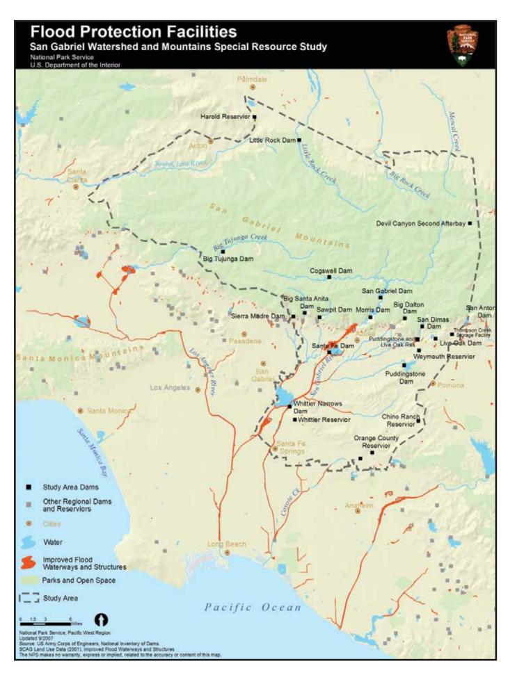
unlined San Gabriel River downstream with large flows continuing to Whittier Narrows Dam. Water can also be diverted just below Santa Fe Dam and routed via Sawpit Wash to Peck Road Spreading Basin and the beginning of the Rio Hondo water conservation system.
