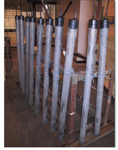
**Photograph 6.** High silicone cast iron anodes used with Alternative B.
