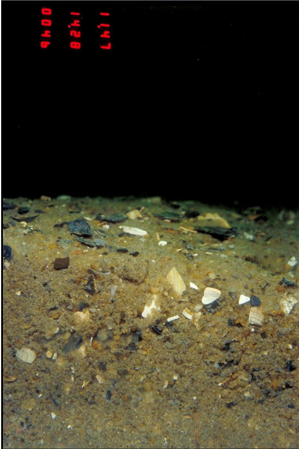
Figure 6-12. Sediment profile image from Station 16, Area 1, May 1998, Survey 1 showing poorly-sorted sediments with shell hash not only on the sediment surface but admixed down to a depth of 7 cm (image width represents 15 cm).
